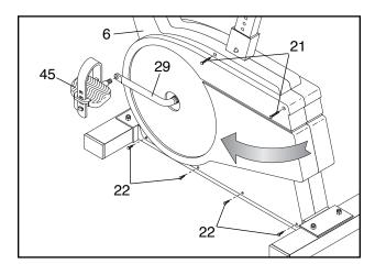
Remove all Screws (21, 22) from the bottom of the Left Side Shield (6). Grasp both Side Shields at the top and gently pull them apart. Make sure that the arm of the Crank (29) is in the position shown in the drawing above. Hold the Left Side Shield at the rear and pull it gently away from the frame. Work the Left Side Shield forward off the arm of the Crank and remove it.
